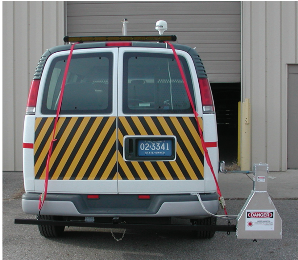
Figure 3.4.9 High Speed Underclearance Measurement System
